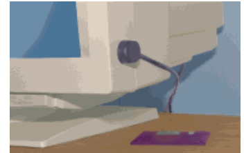
Manual dimmer mounted on computer monitor
